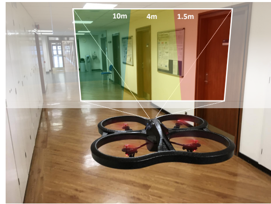
Fig. 1. The proposed regression CNN, trained on our custom dataset collected and annotated in a self-supervised manner, predicts the distance-to-collision towards three directions within the camera’s field of view, based solely on visual input, to navigate autonomously in indoor environments. Supplementary Video: https://youtu.be/43dmXKprIVQ
