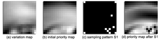
Fig. 2. Learning for sampling patterns: (a) the variation map of the patch location marked in Fig.1; (b) the priority map computed at each pixel by eq.9; (c) sampling pattern (white dots are pixel locations to sample)  $S_1$  at level 1 picks pixel locations with highest priority in (b); (d) updated priority map after  $S_1$ .
