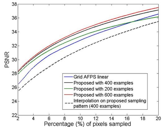
Fig. 4. Performance evaluation with  $q = 99.9\%$ ; for the patch location in Fig.1, 100, 123 and 134 eigenvectors are reserved for 200, 400 and 600 training examples in the database, respectively.
