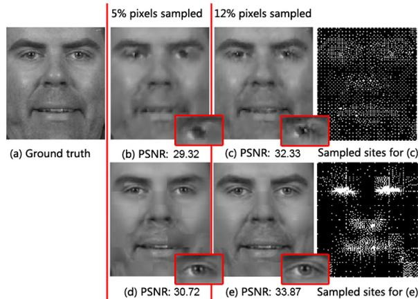
Fig. 3. Example reconstructions with different amount of pixels sampled; (b)(c) are reconstruction examples obtained from global AFPS and triangle-based linear interpolation; (d)(e) are reconstruction examples obtained from the proposed method with  $q = 99.9\%$ . The locations of sampled sites for (c) and (e) are shown to their right side.
