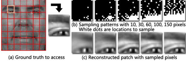
Fig. 1. Patch-based sampling/reconstruction process
