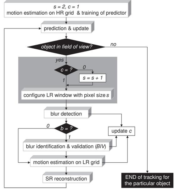
**Fig. 2.** The algorithm of the system operation for a dynamic region.
