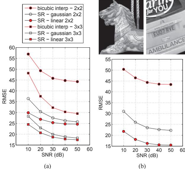
**Fig. 5.** Errors for the two sets of experiments, for various SNRs. The legend applies to both graphs, with (b) containing only the  $2 \times 2$  configuration values. The ground-truth frames are shown at the top.
