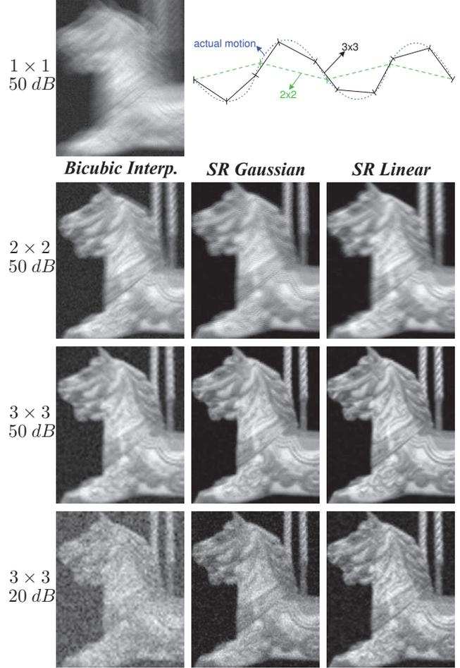
**Fig. 4.** Row 1: The raw output for configuration  $1 \times 1$  (elementary pixel grid), and the intra-frame motion of the time samples produced during HR integration for each configuration. Rows 2-4: SR reconstructed outputs when employing the indicated PSF approximations.
