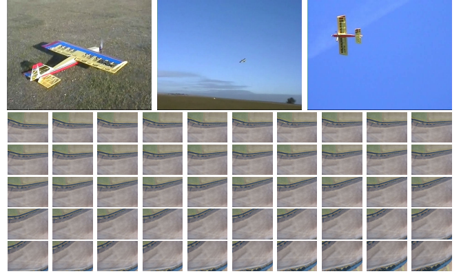
Fig. 4. Setup for real-data testing. The Barnard Microsystems In-View unmanned aircraft is equipped with an on-board digital camera, and the captured video sequence is used in the tests.
